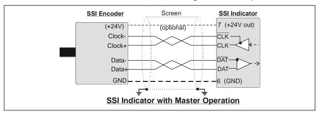
When your encoder receives already its clock from another device and the unit should only "listen" to the communication, then set register "Mode" to "Slave". In this case, both clock terminals (CLK) are configured as inputs.
